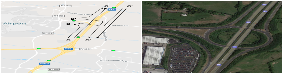
Fig. 3.1 Flow model at the selected intersection in Dublin with six different traffic flows from A to B, A to C, C' to A', C' to B, B' to C and B' to A.
