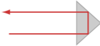
Figure 8 An illustration of the principle of a retroreflector.
