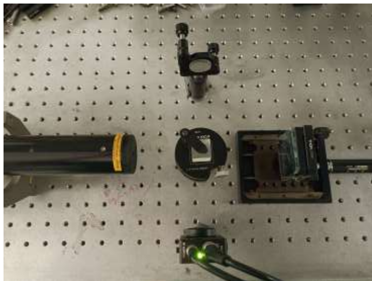
Figure 9 Photograph of the Michelson interferometer type Fourier transform spectrometer used in this experiment.
