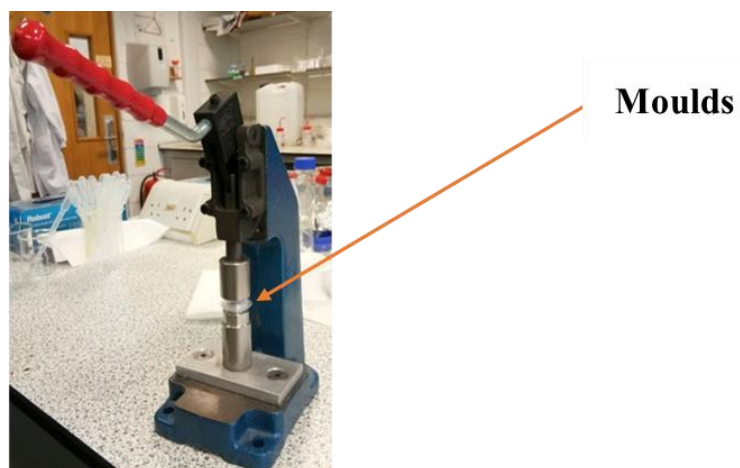
Figure 2.7: Compressor to release cured lens from moulds.
