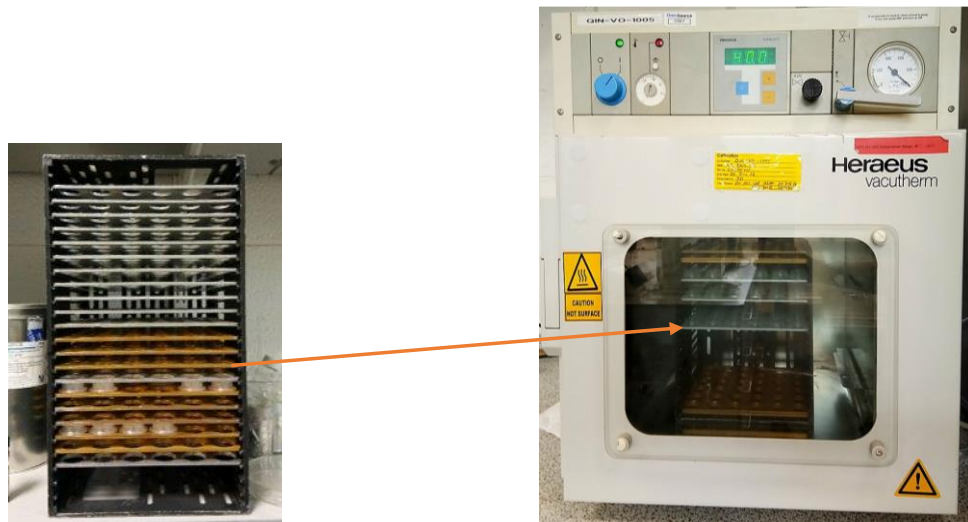
Figure 2.5: Lens mould tower (left) and Heraeus vacutherm oven with mould tower inside (right).
