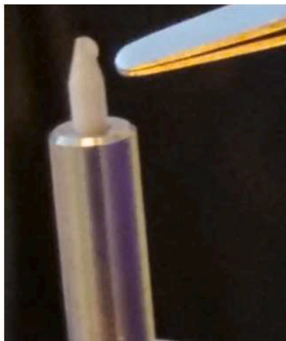
Fig. 10. Build-up of dried dissolving microneedle formulation at the tip of the nozzle.
