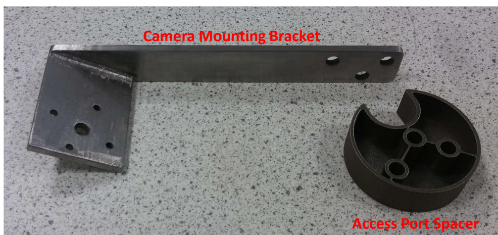
FIGURE 4.22: Designed and manufactured camera mounting bracket and access port spacer.
