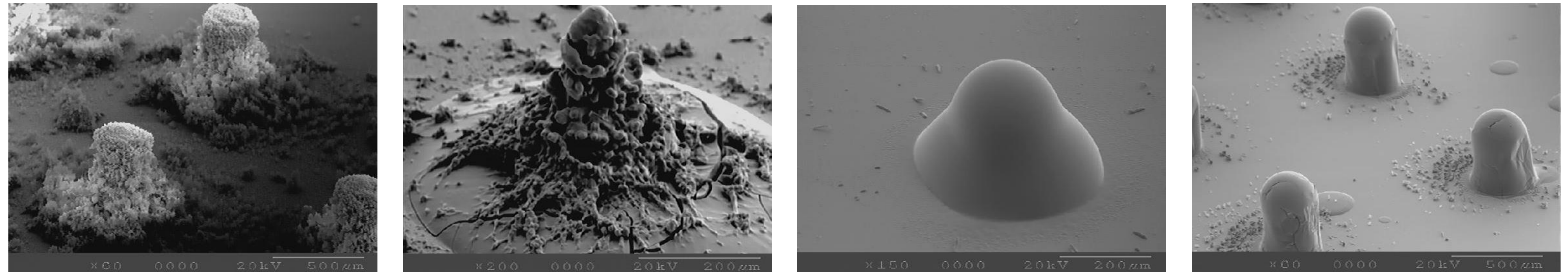
Figure 2: SEM images showing the evolution of printed microneedles during development using Aerosol Jet Printing.
