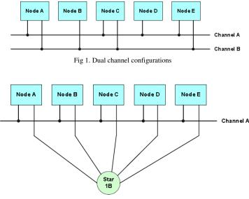
Fig 2. Dual channel implemented as different network types
