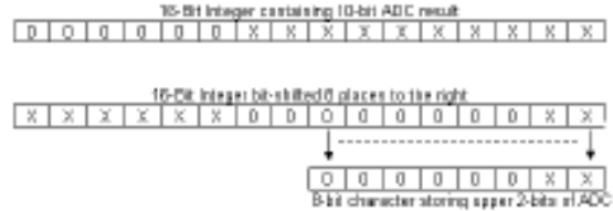
Figure 10: Manipulation of 16-bit Integer to obtain the two LSB's of ADC result
